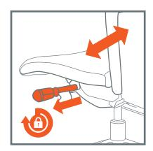
**Synchronised Mechanism** Left hand as seated: 1 handle and paddle
