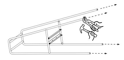
**3.** Hold the nuts with the wrench and remove the screws from the stretcher.
