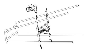
**4.** Remove the 8 screws from the top of the frame.
