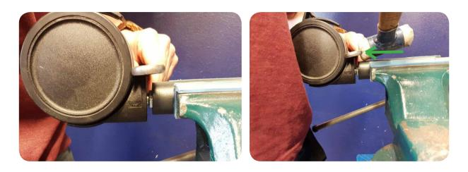
3 As soon as the wheel is out of its locking mechanism, it will easily come off. Be aware that you might need to hit multiple times with the rubber hammer, before this happens.
