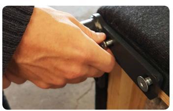
3 Screw the screws loosely in the 4 bottom inserts, using fingers only. Use the other hand to guide the skid frame into correct position for the inserts.
