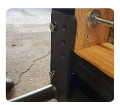
Tighten the screws with a size 5 Umbraco key.
