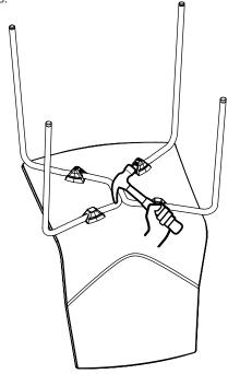
**2.** Use a pipe wrench and a hammer to remove the glides.
